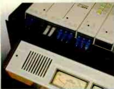
conductive plastic faders and LED lighted switches for reliability. Socketed ICs for fast on site repair.
