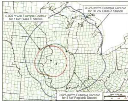
Figure 3: Tell city waiver AM interference contour example
