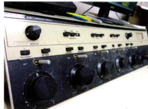
A McMartin audio console still in operation and used for producing stories in the newsroom.
