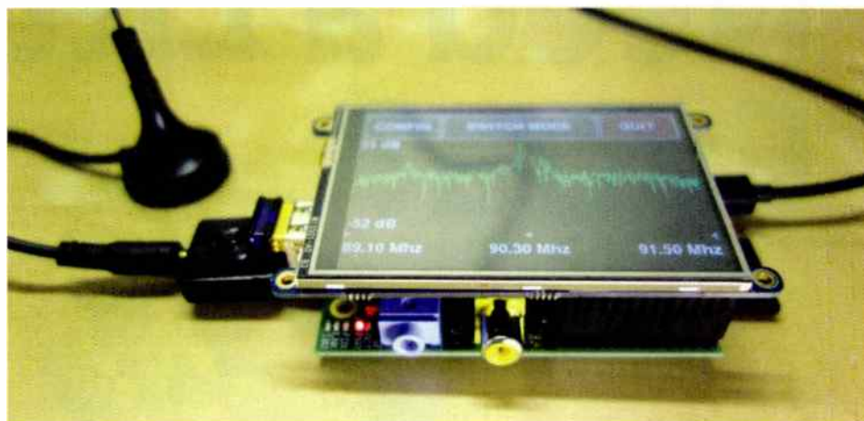
Raspberry Pi as a simple spectrum analyzer with RTL SDR receiver attached via USB.
