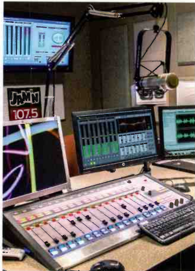
The E-6 surface was chosen on music stations for its EQ and dynamics processing control among other reasons.
