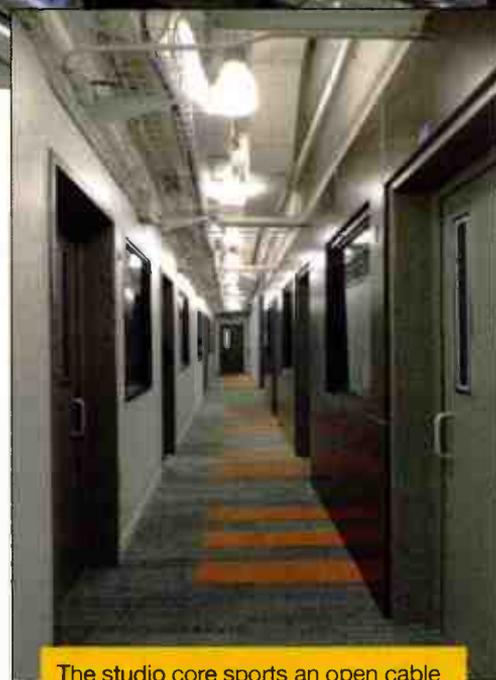
The studio core sports an open cable tray, Industrial Acoustics doors and a straightforward layout, with control rooms and mixing studios on the left, production rooms on the right.
