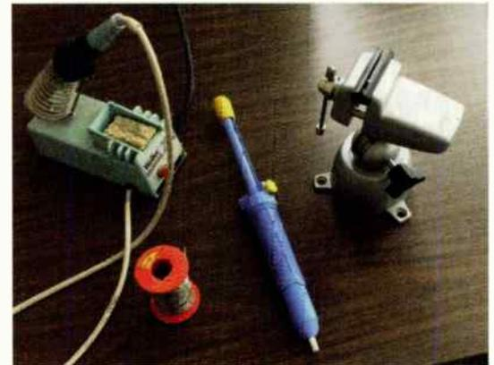
These are the basic soldering tools needed in every engineering shop.
