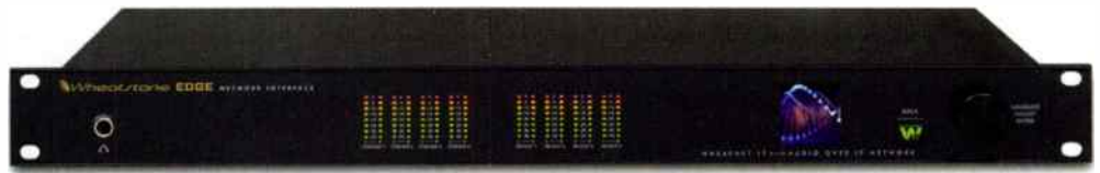
Wheatstone Edge provides the interface between Wheatnet-IP and longer-latency IP networks.
