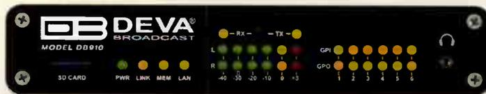
This radio gear is equipped with two-way GPIOs and RS-232 serial communication that could be used for telemetry and automation. The front-panel audio level bar graphs and LED indicators of the unit allow reading the current state of the device at a glance.
