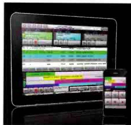
The Simian Gateway creates a TCP/IP portal into your Simian 2.2 & 2.3 Pro automation system for Simian Remote for PC, Simian Remote for iPhone and Simian Remote for iPad clients to connect. The Simian Gateway manages a connection to your Simian 2.2 & 2.3 Pro on-air or production software to Simian Remote clients on your local network, or across the internet.
