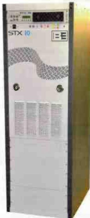
and power supply modules are hot-pluggable and hot-swappable, so there's no reason to take the transmitter off-air to install a spare. The combiner will auto-adjust to the power change when a module is added or removed. Auxiliary power supply options are available for the PA power supplies and controller power supply providing the ideal redundancy configuration. Moreover, the STX10 has a redundant cooling system, allowing it to operate at full power with a fan failure.
