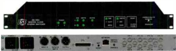
timecodes are monitored and will switch to the backup master clock upon failure of timecode (three selectable modes: ESE, SMPTE-LTC/EBU or either). The ES-150U has LED indicators that displays status of both timecodes and auto switchback or trip (manual reset) mode. If preferred, network control of the ES-150U is optionally available.
