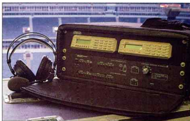
A small field package holds the terminal adapters (top) and digital audio codecs (bottom) used to backhaul 20kHz stereo audio from the stadium over a single Basic Rate ISDN circuit.
