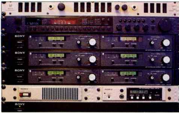
The setup uses frequency-agile wireless microphone systems in the UHF and VHF bands.
