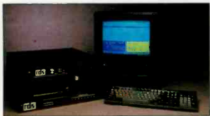
The Phantom from Register Data Systems is an example of an IBM PC-based digital storage and automation system.
