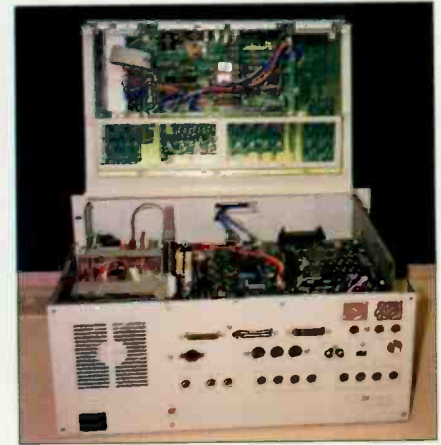
A look under the hood of the Roland DM-80's CPU (rear view). All audio, MIDI and SCSI I/O connectors for the system appear on the CPU's rear panel.
