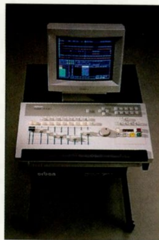
The Orban DSE 7000 is an IBM PC-based DAW with a dedicated control surface that emulates a mixer and a tape transport.
