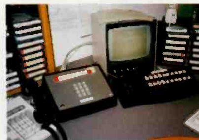
The call screener position is sometimes located in the control room.
