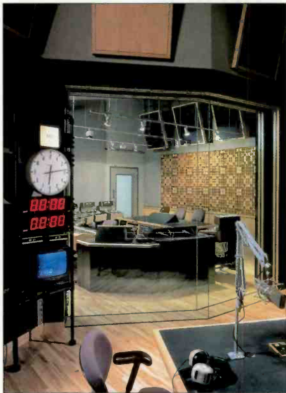
Careful room shaping can allow good sightlines between a control room and studio while still maintaining an optimum monitoring environment. (NPR, Washington, D.C.)
