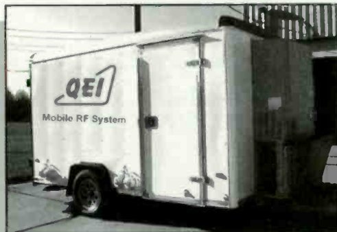
Transportable Pre-Built Transmitter Sites
