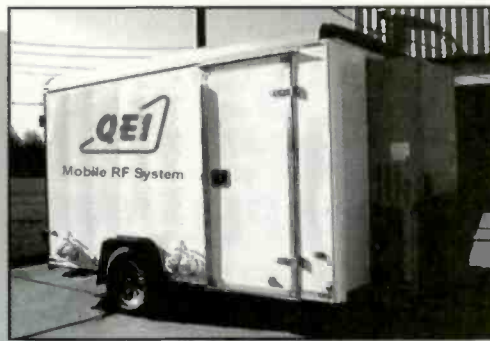
Transportable Pre-Built Transmitter Sites
