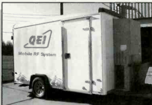
Transportable Pre-Built Transmitter Sites
