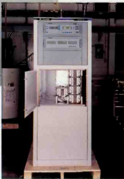
A clean and simple layout makes servicing the Z5CD much easier. The amplifier modules pull out for easy maintenance.
