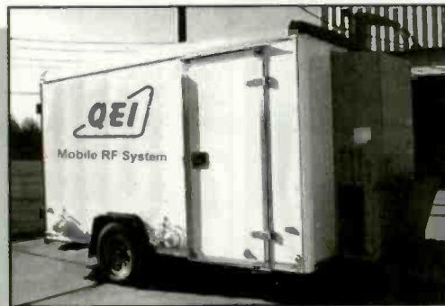
Transportable Pre-Built Transmitter Sites
