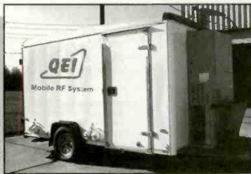
Transportable Pre-Built Transmitter Sites
