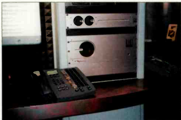
New breeds of on-air telephone systems that use ISDN and T1 carriers are being introduced.
