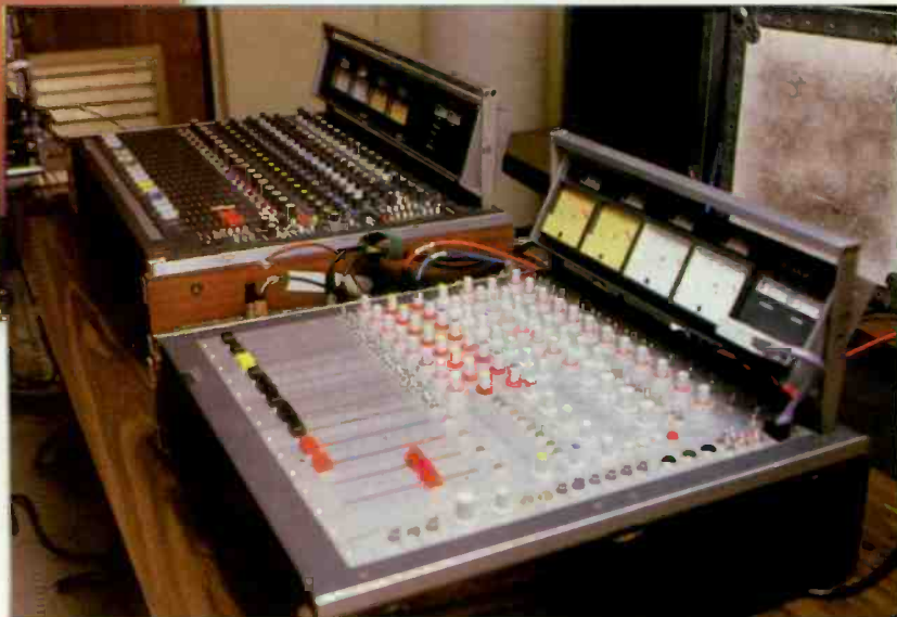
For the Chamber Music Society broadcasts, a 16x2 console is linked to an 8x4 console.
