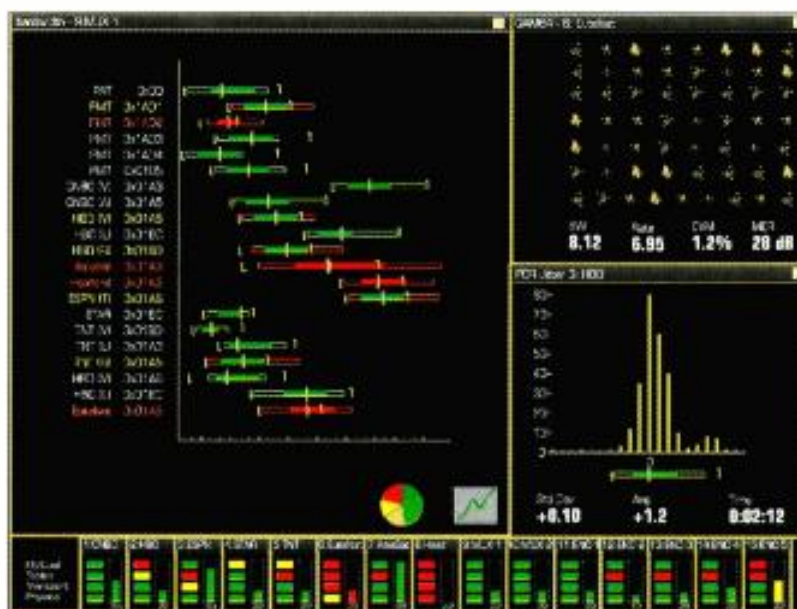
Pixelmetrix's DV Station reports multiport correlated status of physical, transport, coding, and quality layers.
