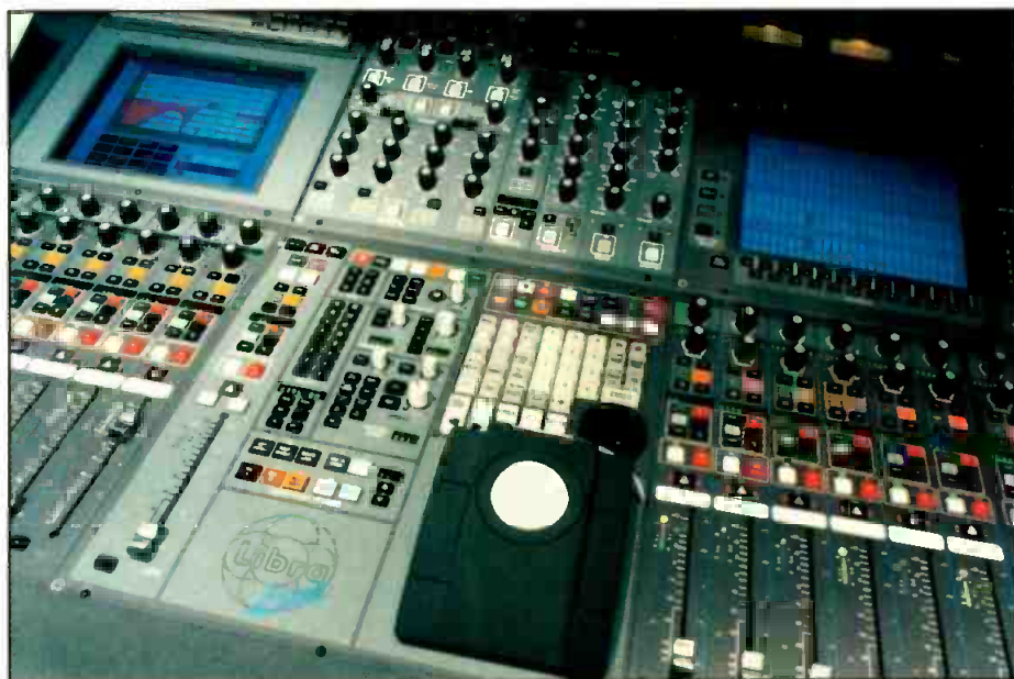
Automation and the ability to be customized to meet individual engineers needs are the biggest advantages to digital audio consoles. An AMS Neve Libra Live audio console is shown here. Photo courtesy of AMS Neve.
