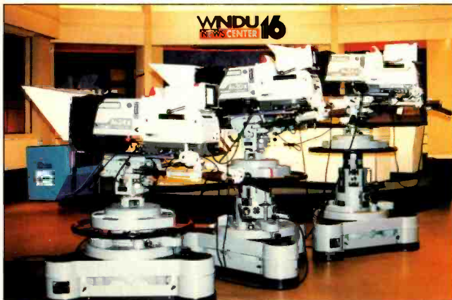
WNDU-TV/DT selected Ikegami's HDK-790D cameras to capture images in both 4:3 NTSC and 16:9 HDTV formats. The decision allows WNDU to meet its current goals and prepare for the future needs of its two studios.
