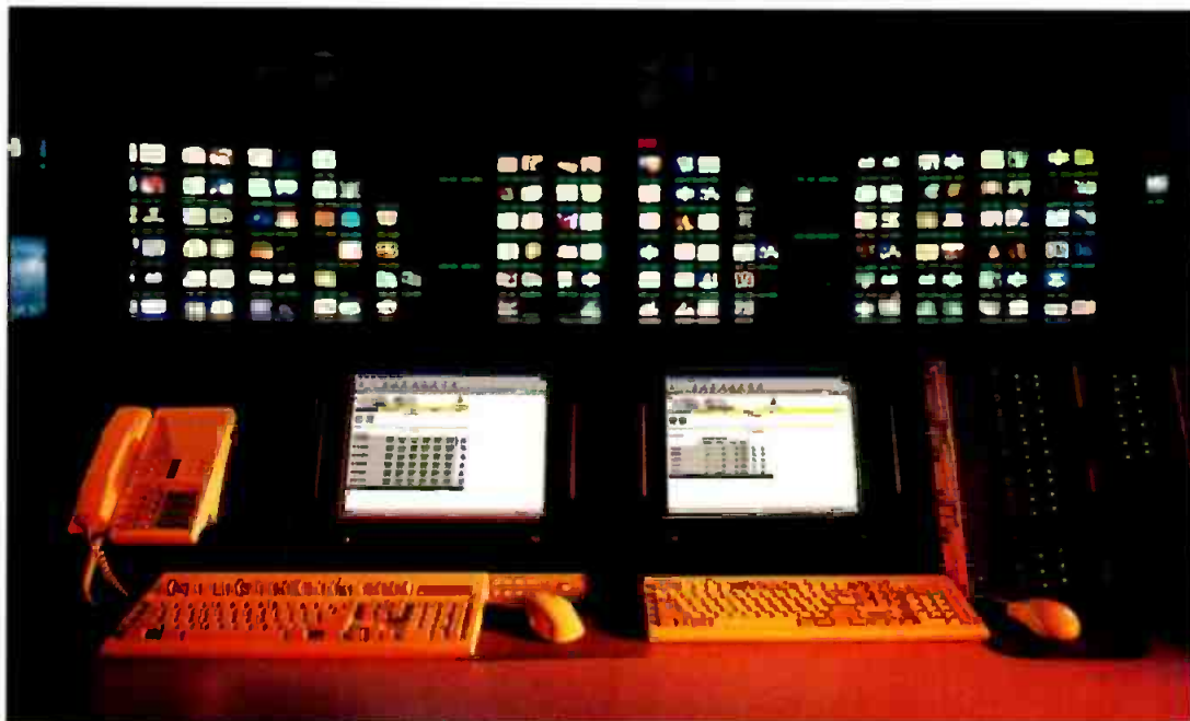
At its state-of-the-art Uplink Center in Cheyenne, WY, EchoStar uses the Acterna DTS-400 MPEG-2 digital broadcast monitoring system to monitor all 500 of DISH Network's primary services.
