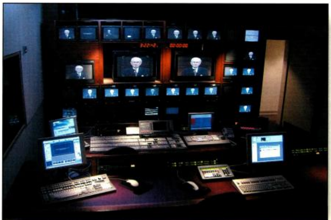
One of two virtually identical Video Production Control Rooms. Room 1 is high definition, Room 2 is standard definition. Both rooms feature Sony BKDS7026 and HDS7000/DVS7250 production switchers with HDME700/DME7000 DMEs.
