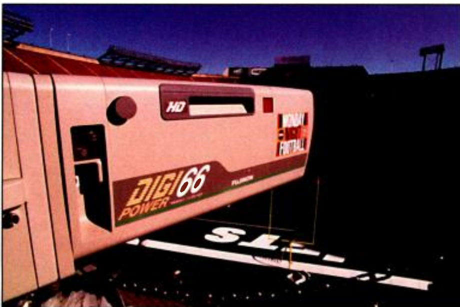
Camera Four, shown here at the Meadowlands in East Rutherford, NJ, is situated behind the end zone and mounted on a tripod high in the stands. Camera Four is a Panasonic AQ-7200 studio camera with a Fujinon HA66x9.5 BESM high-definition lens.
