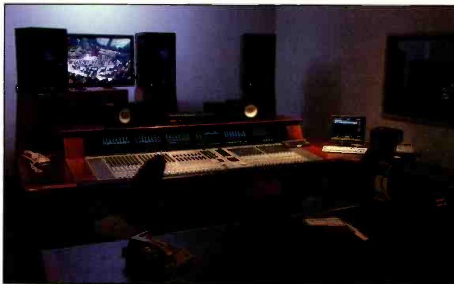
The Euphonix C-5 systems in the two Production Audio Control Rooms provide a base from which all originating sources can be 24-bit and support up to a 96kHz sampling rate for live and post production.
