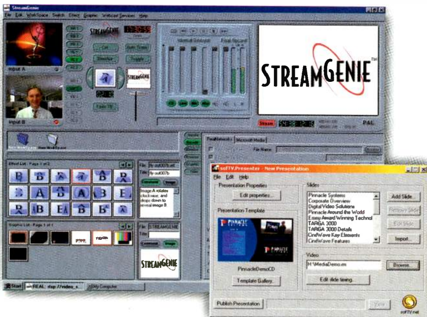
Encoders like the Pinnacle StreamGenie, shown above, allow broadcasters to reach larger audiences on the Web by encoding streaming content into multiple formats. Photo courtesy Pinnacle Systems.
