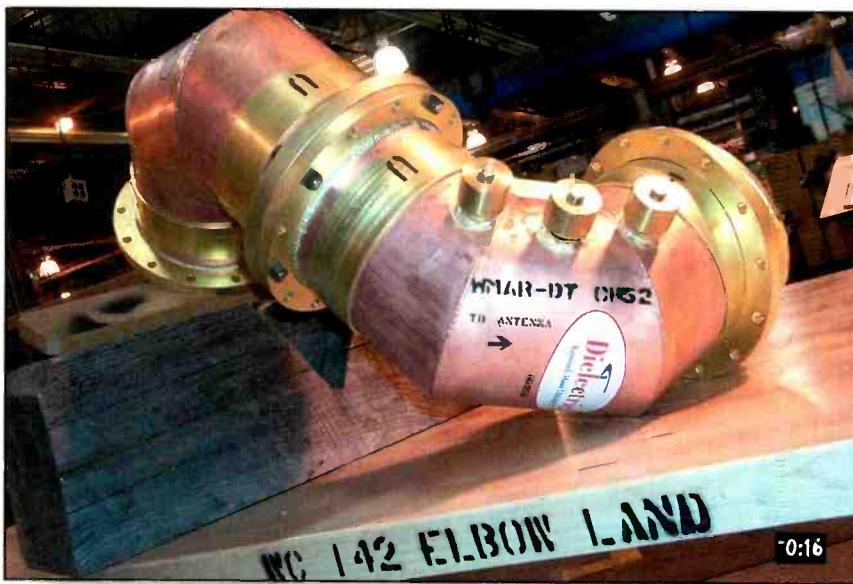
Especially at the top of the tower, elbows are often connected back to back, as shown above, which can cause mismatches in the signal. Photo courtesy Dielectric.
