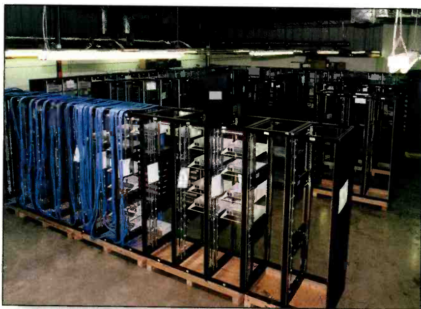
Off-site prefabrication of rack infrastructure ensures both equipment compatibility and a good fit, thereby helping to eliminate last-minute snags.
