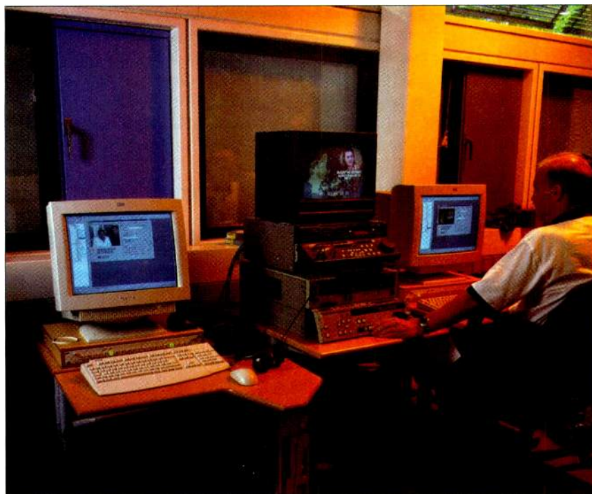
A Danish Broadcasting operator is performing ingest using Keyvia's (formerly Keops) Key-MediaWorks – creating and checking in multi-resolution assets to the asset management system from VTRs and satellite.
