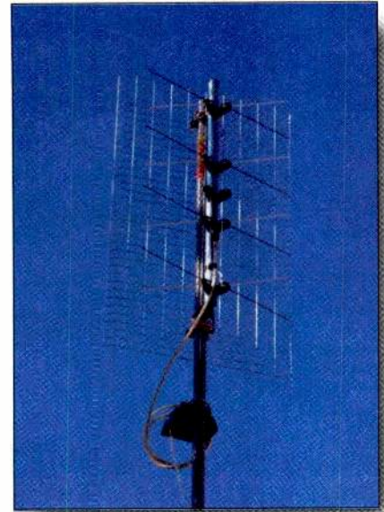
As I experimented, I found that classic antenna designs often worked better. This antenna design is nearly 50 years old, but it's fine for UHF DTV reception.
