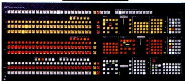
Early digital production switchers have evolved into versatile live production tools, many featuring internal digital effects, increased inputs and programmable outputs. Zodiak from Grass Valley Group is shown above.
