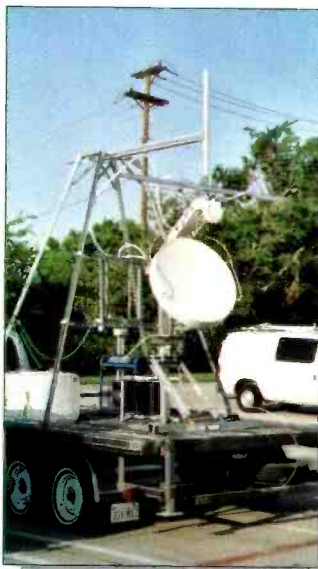
Tests performed at Andrew using the setup above have shown that signals on Ka-band antennas may experience significant degradation under wet conditions. The material chosen for the reflector may minimize this loss.
