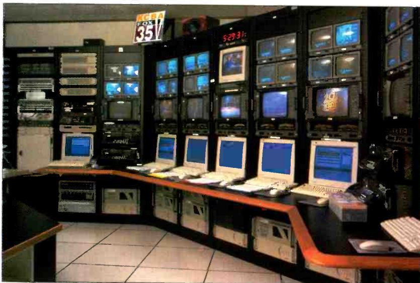
Sundance Digital's FastBreak automation system at KCBA in Salinas, CA, as part of a centralcasting solution. Broadcasters generally should choose an automation system based on the unique needs of their operations. Photo by John Lanning.
