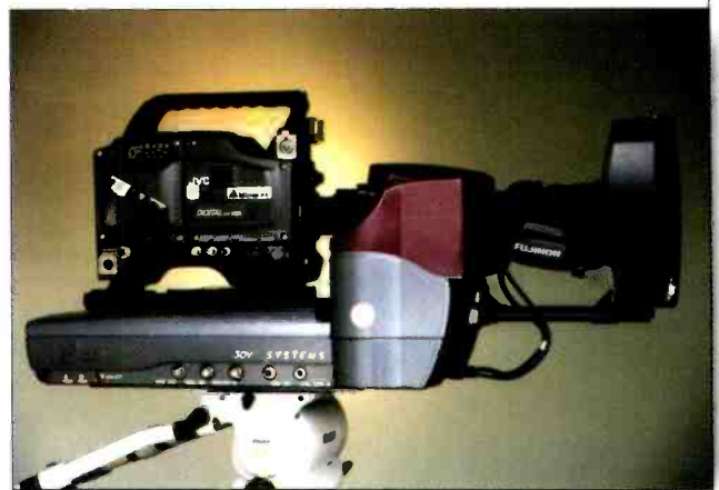
By integrating its 3-D imaging concept with a conventional studio camera, 3DV Systems created Zcam, an RGBD studio system that can separate the background and add/subtract image segments in real time.
