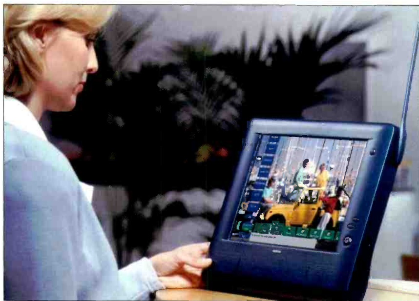
The Nokia Mediascreen is a portable/mobile DVB television and data receiver.
