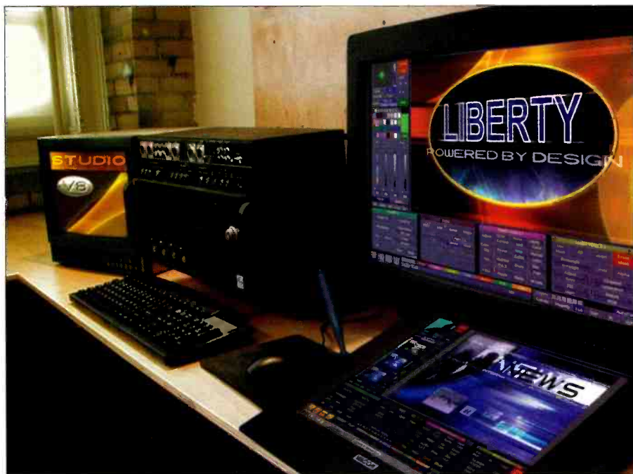
The Liberty Reality Studio is a graphics creation system that integrates Liberty's paint, animation and compositing software with Leitch's dpsReality DDR. Operators have the ability to capture video material, create and add graphics, composites or animations, and then output directly to other record and playback devices.
