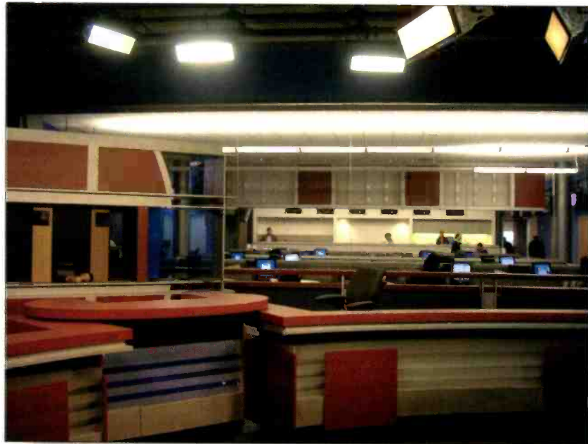
Stations can fulfill the NC 25 requirement of a TV studio by using glass to separate the studio from newsrooms and other technical areas.
