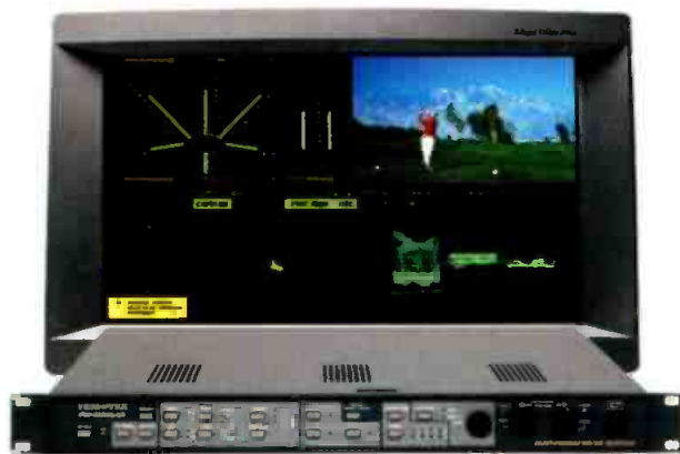
Sophisticated combined displays can be created by digitizing the signal and displaying the results on a computer monitor. Photo courtesy Videotek.
