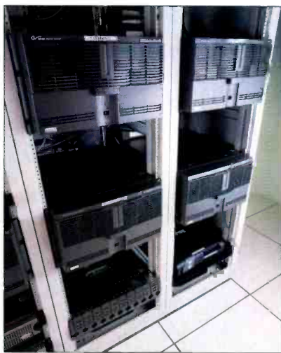
WLS-TV chose SCSI Fibre Channel-connected Thomson Grass Valley Profile XP media platform servers.
