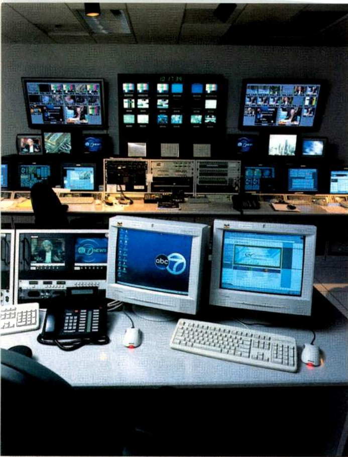
The large monitor walls in the WLS-TV newsroom allow the staff to monitor multiple incoming signals, as well as the competition, all at once.
