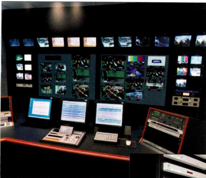
The Miranda Oxtel Imagestore at the master control room at WHRO incorporates all the functionality required in a master control chain in a single box, including AB mix, four key layers, logo generator, character generator, DVE, still store, clip-playout server, audio mix, audio store and EAS insertion. Photo courtesy of CEI.
