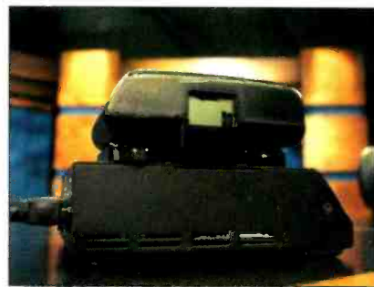
Modern batteries communicate digitally to chargers like the Anton-Bauer Dual 2702 Powercharger shown above while talking to the user through an LCD window.
