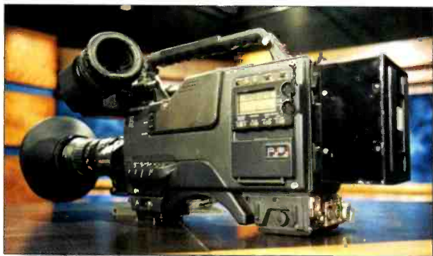
Cameras have shrunk while lenses and batteries have kept their size and weight, allowing each to balance the other. Without rear-mount batteries, smaller cameras would be front-heavy, and on shoulder-mounted cameras, balance rather than weight is the critical factor.
