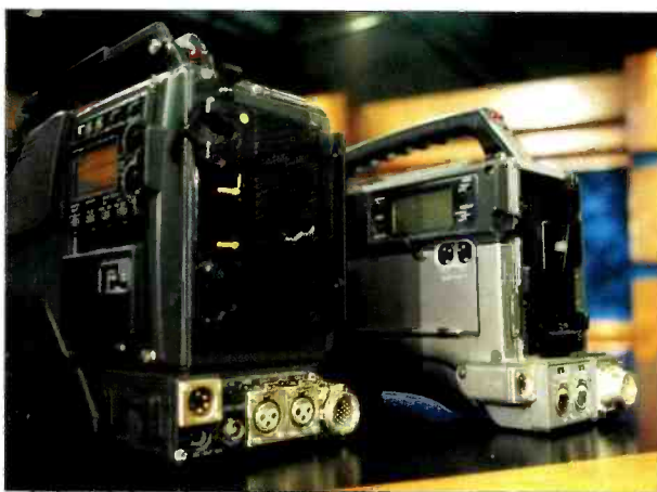
This photo shows the two most common camera battery mounts. The camera on the left has the Anton-Bauer Gold Mount. The other has the Sony V-mount.
