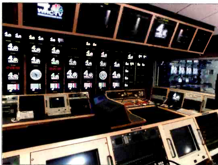
The WRC production control room in Washington, DC, is built around a Grass Valley 4000 switcher, which allows up to 64 inputs for video and/or keying. Photo by Felix A. Peña, director of mechanical and computer services for CEI.
