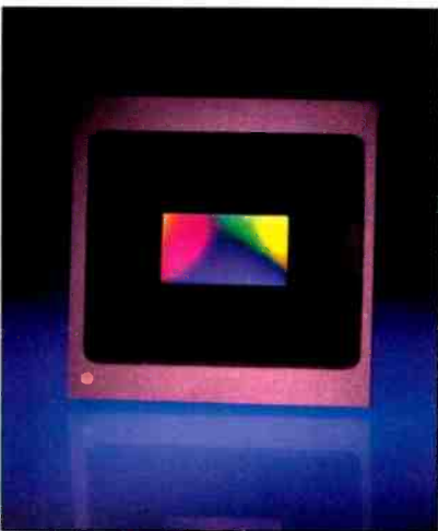
This photo shows the ProCamHD 3530 CMOS image sensor in a standard 65-pin PGA package. Three such sensors are incorporated into the new HD cameras being developed by JVC and Ikegami.
