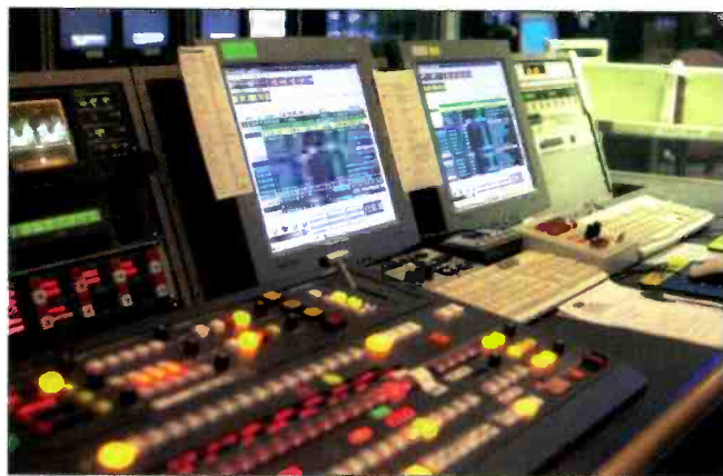
Crispin's System 2000 automation provides a common control point for news and programming, leading to greater efficiency. Upgrades to the system also provided the ability to balance two daily news shows.
