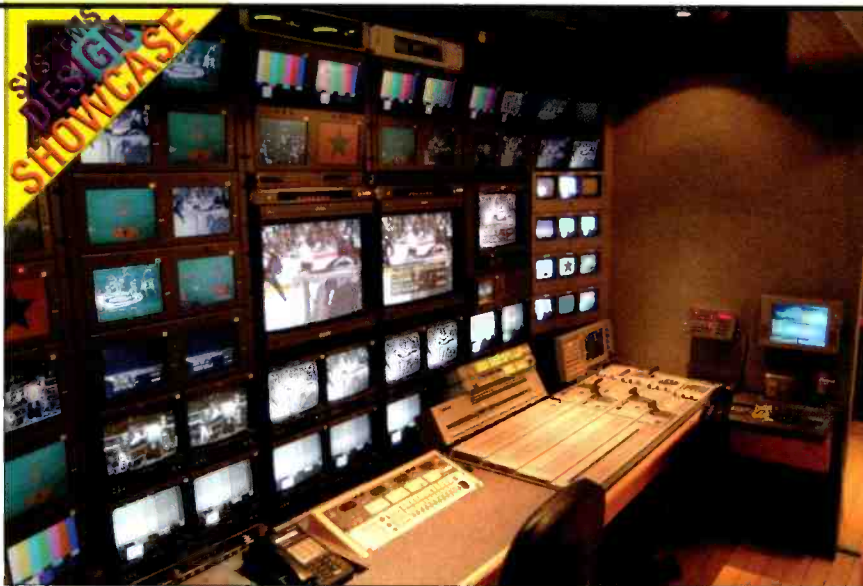
The production room's expansive video wall is all patchable with a full 3.5M/E Sony 7350 switcher and two-channel Sony DME 3000 DVE.
