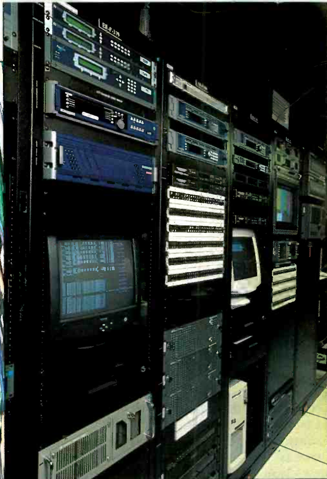
Several Snell & Wilcox Ukon universal conversion platforms and numerous IQ modular systems are used in the equipment room Studio 6A at NBC Studios in New York (left). The Ukons downconvert up to 45 incoming video signals, while the IQ enclosures contain digital audio delay modules for audio/video synchronization. Ukon universal conversion platforms (right) are also used in NBC Studios' network transmission area for upconverting the network feed to prepare HD signals for transmission to affiliates.
