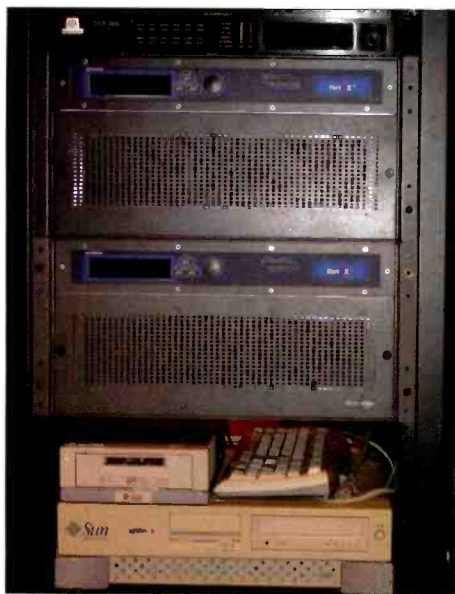
NetVX supports WSU's existing DS-3 microwave transport and helps carry one NTSC and two ATSC program streams to each of the university's transmitter sites.
