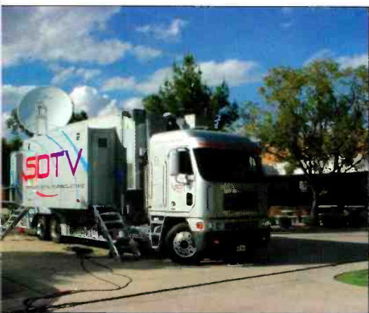
SDTV's ExpandoLink was designed to provide production and transmission capabilities — including eight cameras, 40 channels of audio, and analog and digital satellite uplink — in a 40-foot layout.
