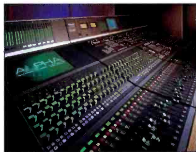
All Calrec consoles incorporate both stereo and mono down-mixing capabilities. Shown here is the Calrec Alpha 100.
