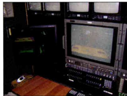
This video shading area uses a multi-display rasterizer for video QC monitoring.
