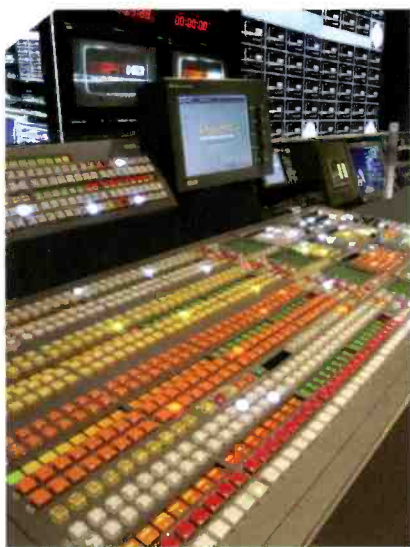
The Thomson Grass Valley Kalypso Duo is an SD production switcher that can be upgraded to HD when required.
