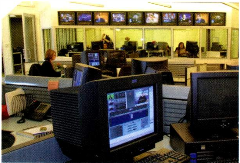
Proxies, in the form of low-resolution video clips and thumbnails, are the index tool that reporters, producers and others use to find the asset they seek with a DAM system.
