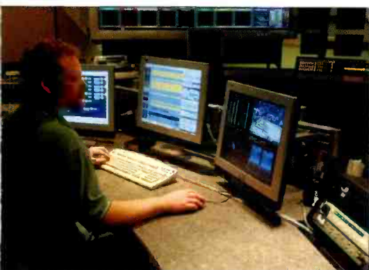
At the pod console, a supervisor can make changes to the air playlist and correct problems reported by a network monitoring operator.
