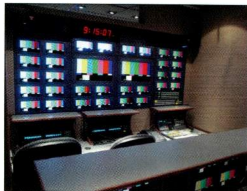
Flat-screen implementation allowed this entire second production room to fit within the standard large-truck footprint of Mira Mobile's recently completed unit.
