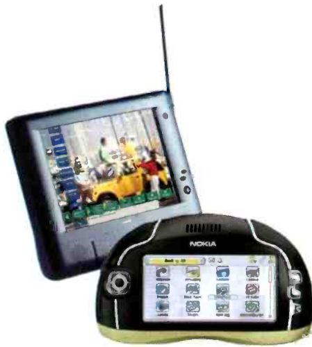
The Nokia DTB-T Mediascreen (left) has a battery life of 20 minutes, while the Nokia 7700 DVB-H Mediaterminal (right) has a battery life of two hours.
