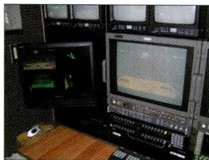
This video shading area uses a multi-display rasterizer for video QC monitoring.
