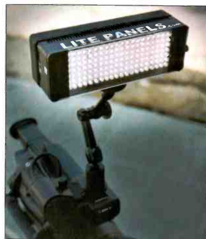
LEDs provide a smooth daylight source that is frugal on power yet packs a surprising punch. The Israeli Arm's single knob permits easy positioning of the light to eliminate eyeglass reflections or the shadow from a matte box.
