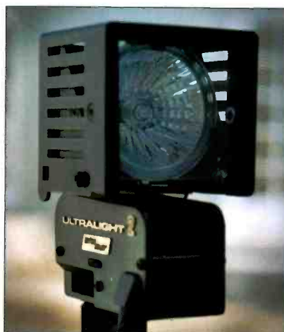
Though lacking in control and subtlety, this on-board tungsten-based unit has been a popular choice for years.
