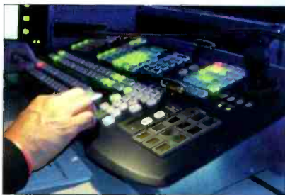
Snell & Wilcox's 1-ME Kahuna sidecar enables operators to do a separate line cut.
