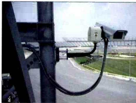
The Vinten HS-102 pan-and-tilt head is positioned discreetly over the track.
