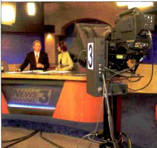
The unmanned camera is controlled by an operator in the control room using Telemetrics' CPS-ST-S control software.
