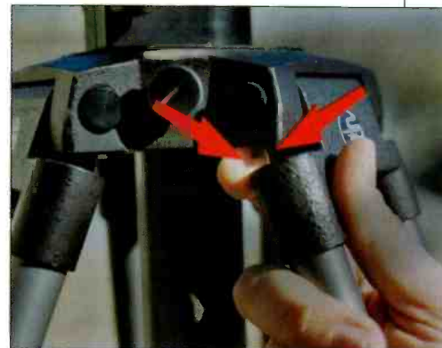
Some tripod legs can cause serious injury. Make sure the people you work with are aware of the potential harm.
