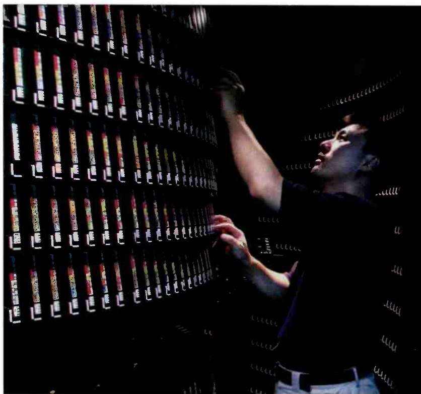
China Central TV's online robotic archive operation consists of a StorageTek PowderHorn 9310 tape library with five T9840B and five T9940B tape drives.
