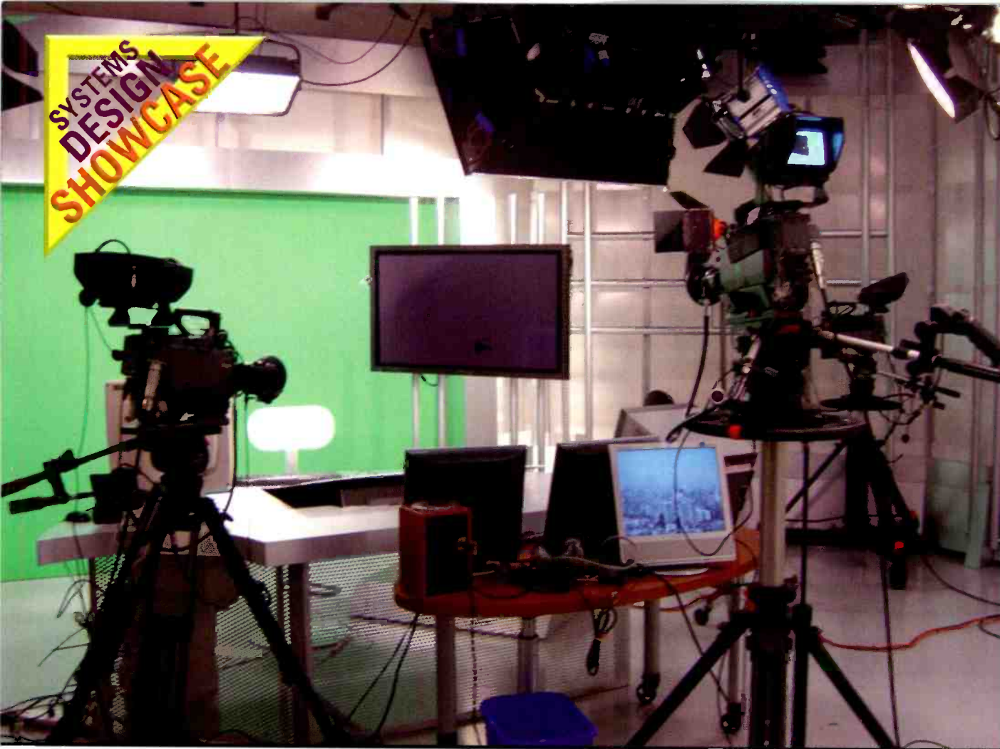
RAI's main production studio features Sony BVW-550 digital studio cameras, while field acquisition is done with Sony XDCAM PDW-510 cameras.
