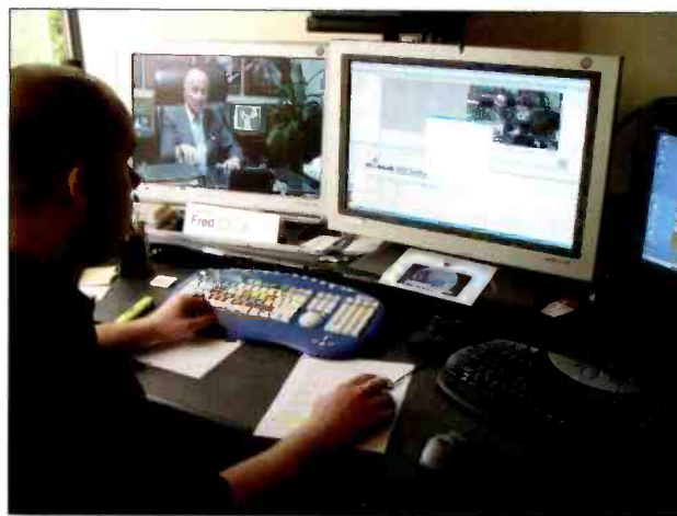
A computer feeds video from an editing system on the SAN to a Grass Valley broadcast system.
