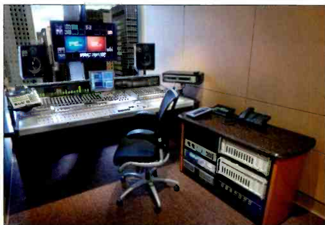
The new audio control room for Court TV features a Wheatstone D 5.1 audio board.
