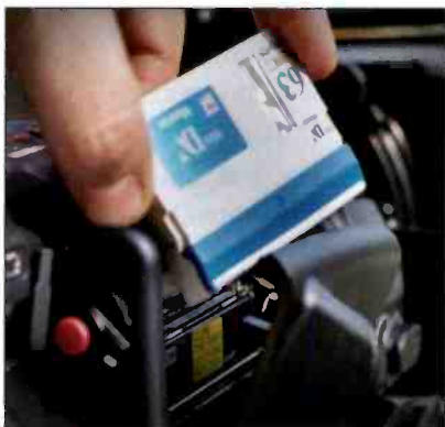
The AG-HVX200 operates as a superb standard-definition DVX camcorder, recording consumer DV 4:1:1 (not HD!) to tape. The 16:9 HD imager contributes an enormous amount of fineness to the SD image — a valuable consideration for ultimate output to standard-definition DVD.
