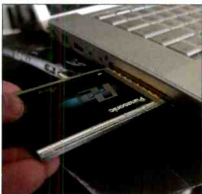
The P2 card may be inserted directly into a laptop, permitting immediate access to footage without capturing. The P2 PCMCIA card mounted on the desktop enables file transfers at speeds theoretically up to 640Mb/s!
