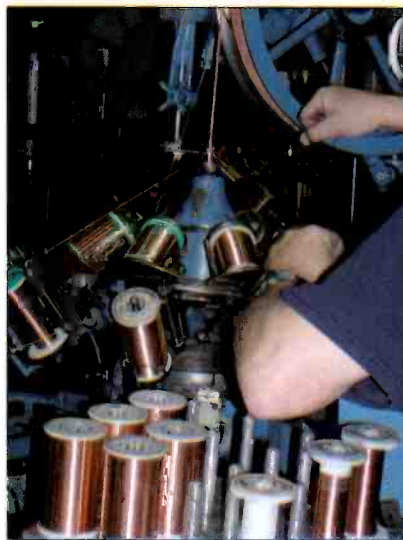
Braiders, mechanical knitting machines, have been around for more than 100 years and are an efficient way to create a woven shield outer conductor.
