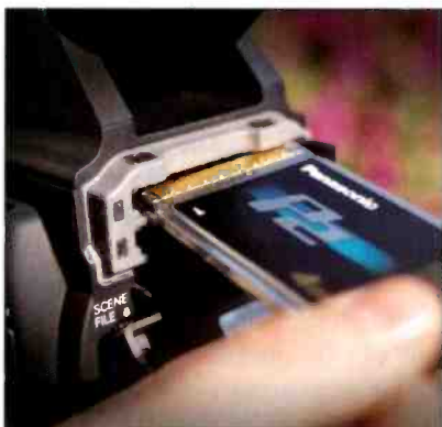
The AG-HVX200 accommodates two P2 cards of 4GB or 8GB each for up to 40 minutes runtime at 720p24pn (native mode). The card not being recorded to can be off-loaded to a laptop, dedicated Panasonic 60GB P2 store, or generic Firewire or USB 2.0 hard drive.
