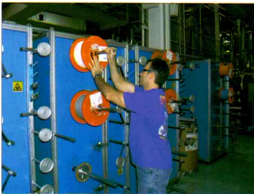
Single-fiber reels are loaded onto a manufacturing line to create a multi-fiber cable. Photos courtesy CommScope.
