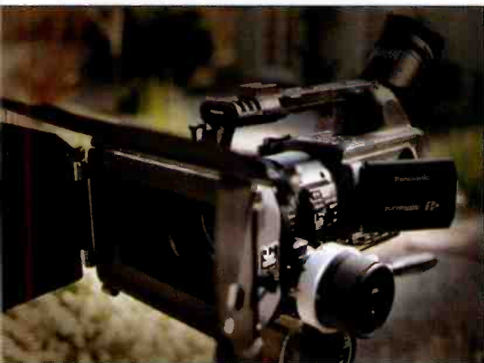
The P2-based AG-HVX200 is shown here with the Chrosziel 16x9 matte box and follow-focus for EFP applications.
