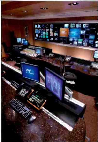
The new Court TV control room uses 4M/E Grass Valley Kalypso switcher.
