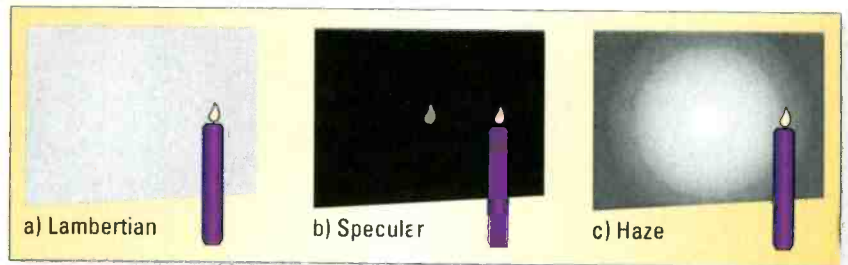
Figure 4. Reflection mechanisms: a) Lambertian or diffuse, in which incident light is reflected in all directions, b) the mirror-like specular reflection and c) haze, with fuzzy circles around the reflected image.
