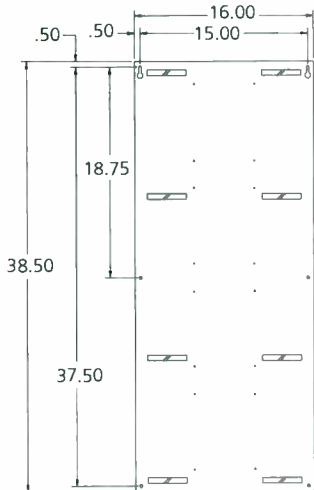
IW-VI-24 24 position, BNC, Bulkhead panel
