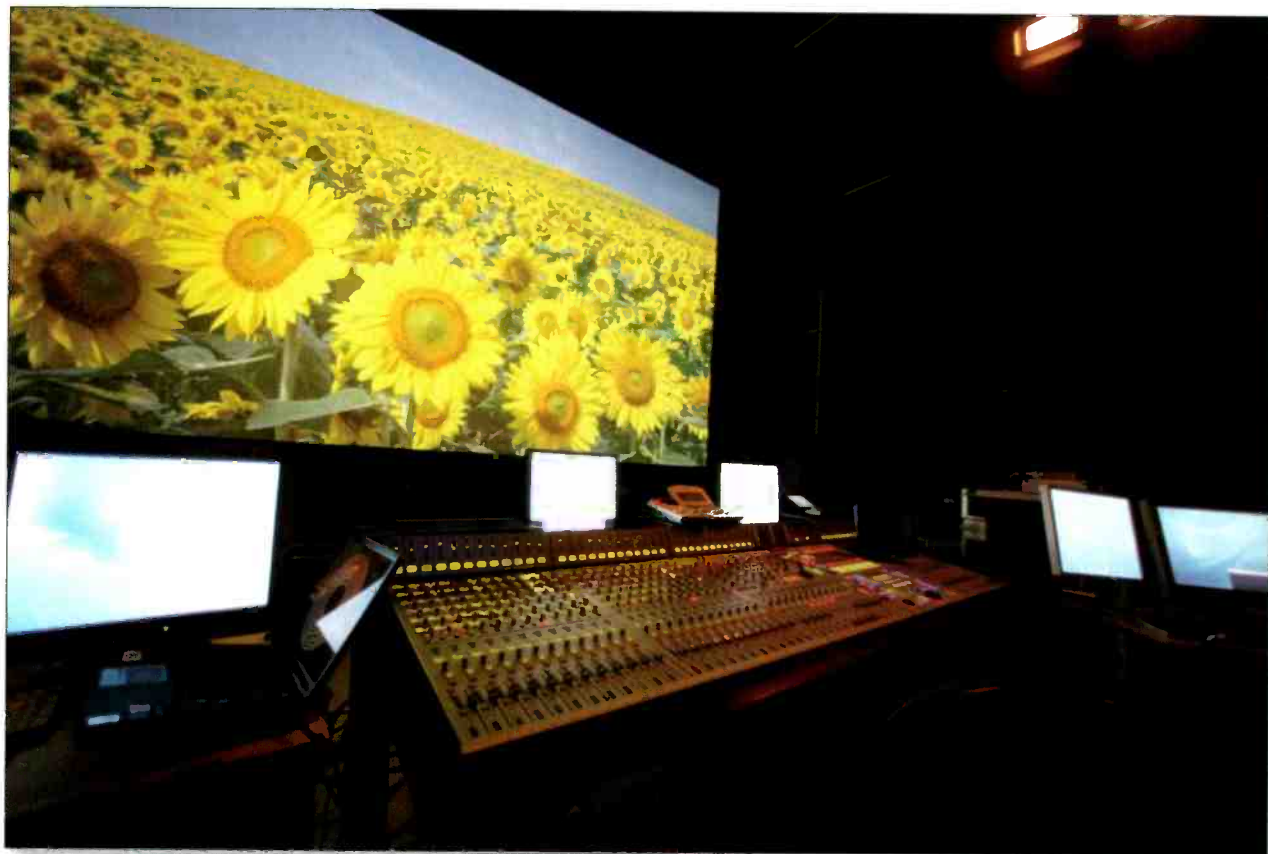
The Fairlight Constellation XT console at NHK lab offers the flexibility needed for a 22.2 multichannel sound system.
