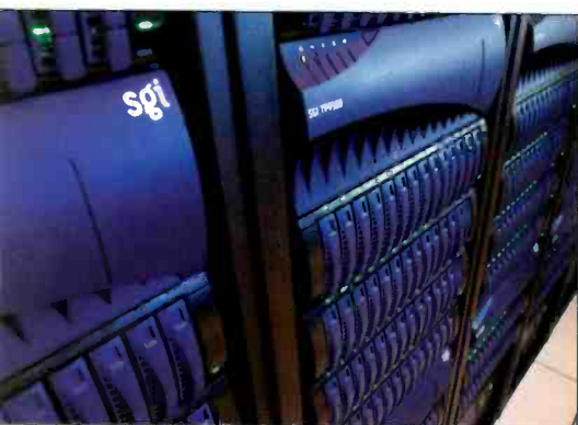
Parallel processing and workflows are enabled by SGI CXFS-based metadata servers designed to power the heart of the I/O and SGI TP9500 storage.
