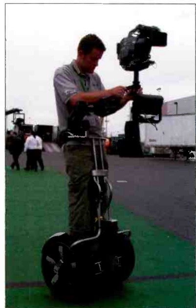
In the outdoor ENG area, HandsFree Transporter's modified Segway turned quite a few heads as a camera-transport system for Steadi-Cam use.
