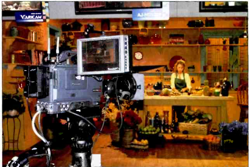
Panasonic highlighted several new cameras in their booth including the multi-format AJ-HDX900 HD camcorder. Recording at 100Mb/s, the HD images are captured in any of 11 video formats, covering both 60Hz and 50Hz platforms.
