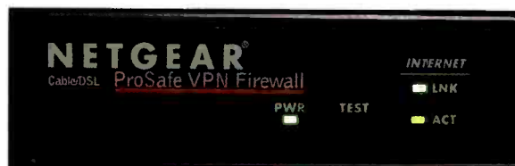
Figure 1. Link and activity lights can tell you a lot about the connection between two network devices.
