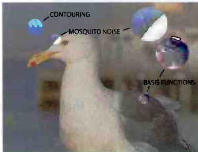
Figure 4. Highlighted here are the three main compression artifacts.
