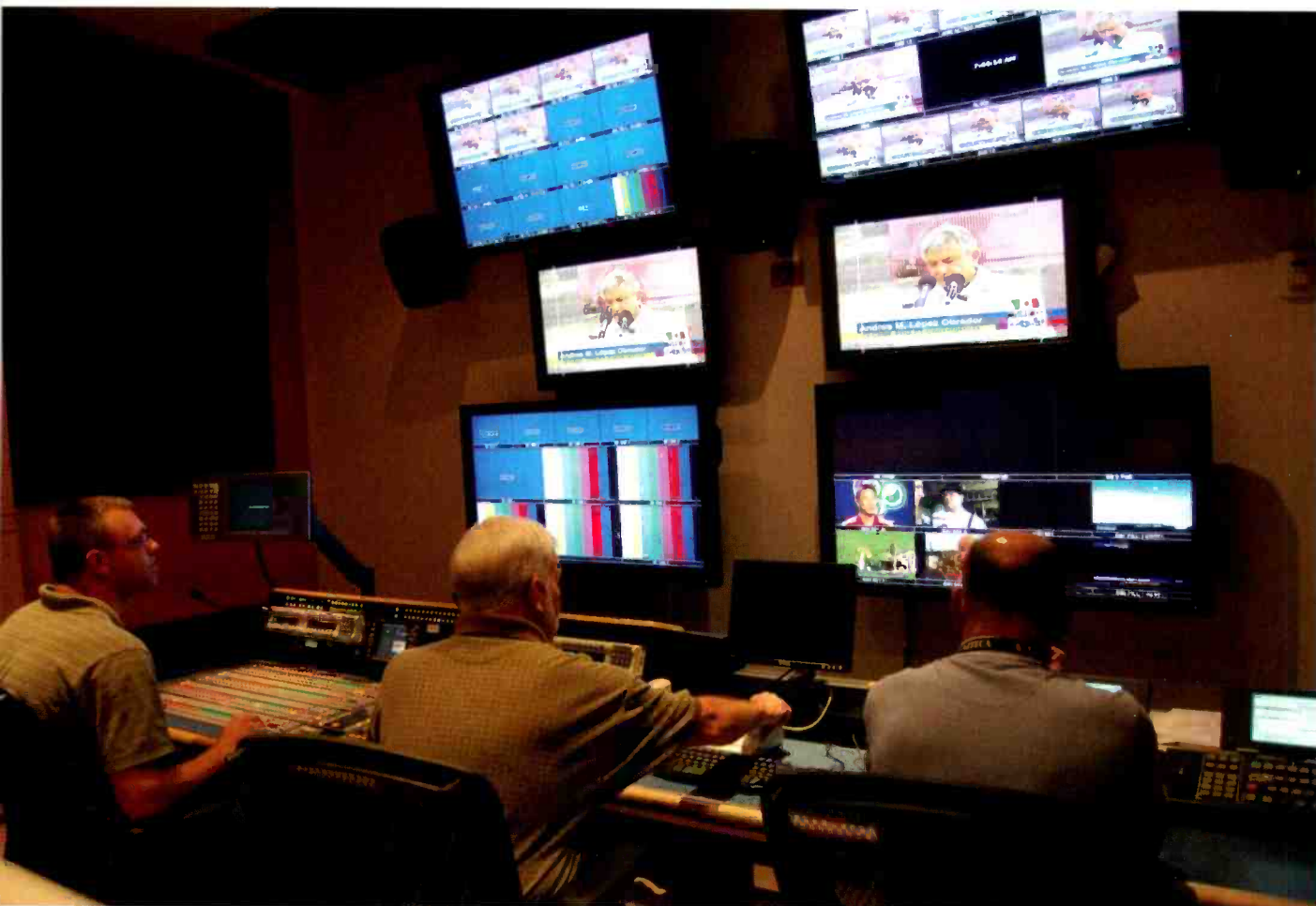
The new HD production control area includes an NEC virtual monitor wall and a Sony MVS-8000 series switcher that supports six cameras.
