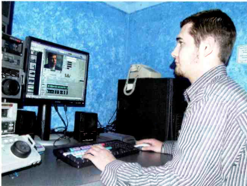
Kevin Fowler, an editor at KTUU in Anchorage, AK, edits an on-air promotion piece using a computer equipped with a Blackmagic DeckLink card and Thomson Grass Valley's NewsEdit SC. Edited material gets sent to playback server system. The output of the system is monitored by the HDLink in another part of the building.
