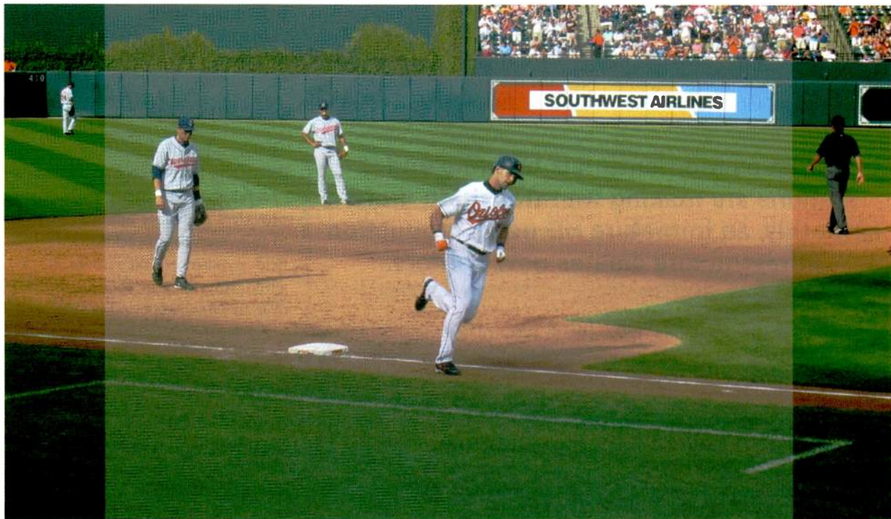
Figure 3. An example of a 4:3 center cut from a 16:9 source. Courtesy HD Consulting.
