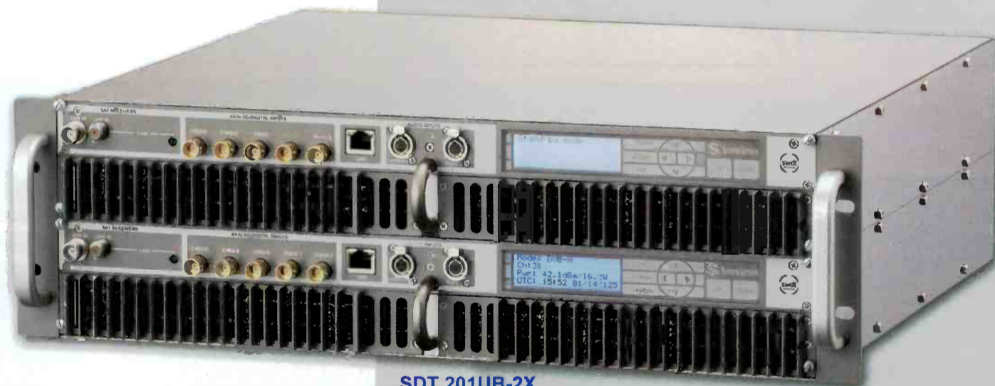
SDT 201UB-2X 3 Units rack 19" On field upgradable 1+1 built-in redundant change-over. 80 + 80 W rms DVB-T/DVB-H 100 + 100 W rms ATSC 200 + 200 W ps PAL/NTSC
