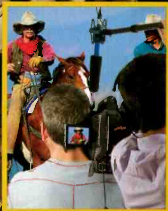
3.5" LCD monitor at rear facilitates audio monitoring
