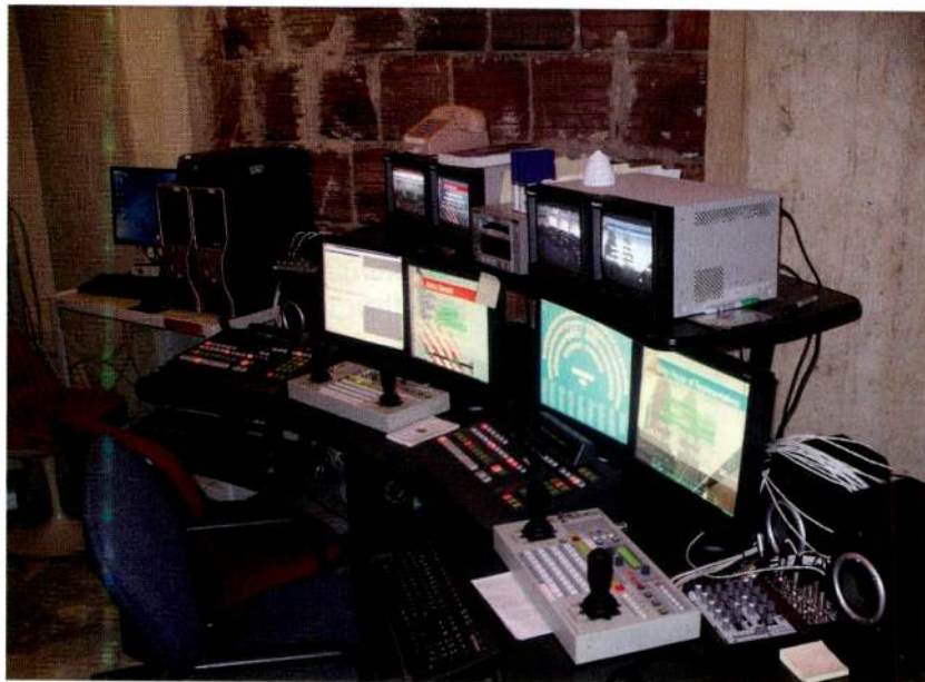
The Slate switchers in the "Legislative Live" control room at the capitol building allow one person to manage switches, call up graphics and work other gear.
