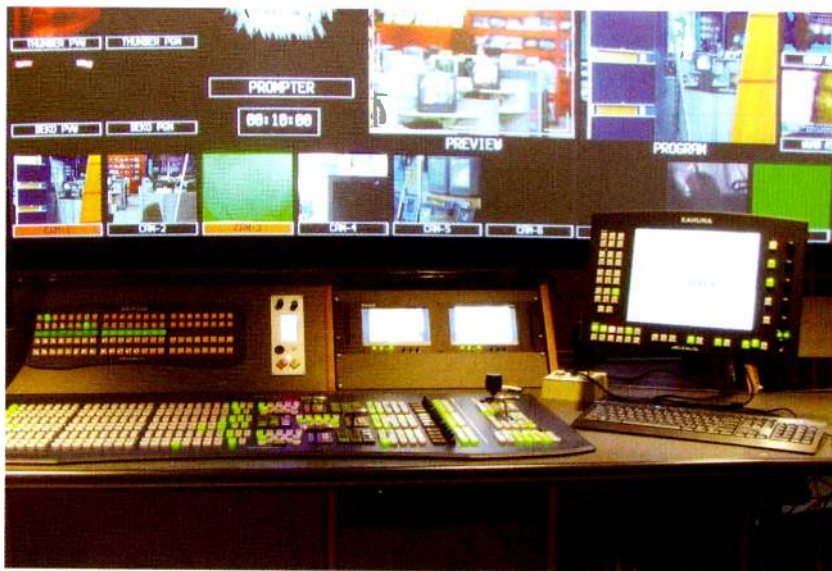
WOIO-TV in Cleveland uses Snell & Wilcox's Kahuna for live news production. The switcher offers simultaneous SD/HD operations in the same mainframe.
