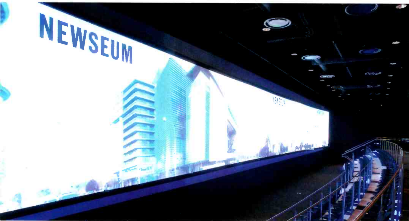
The Big Screen Theater features a 10ft x 90ft screen displaying images from five blended Christie DW3K 720p HD projectors.
