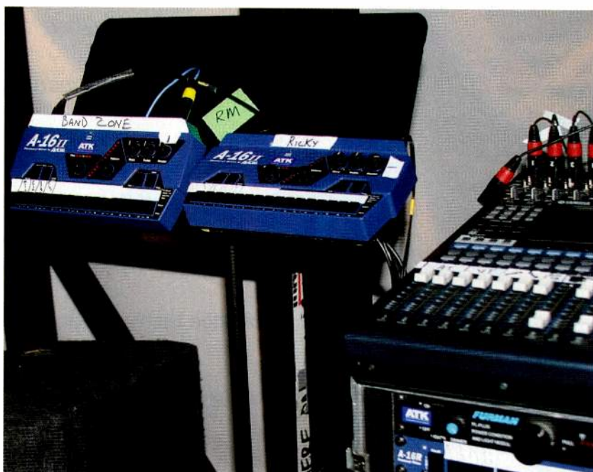
The band's drummer uses Aviom's A-16II personal mixer, which he can control himself. In addition, several other band members use the mixer for monitor control.
