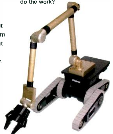
2. The iRobot Warrior x700 can shoulder 150-lb payloads and tackle heavy-duty applications.
