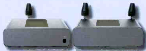
2. The Gefen HDMI Extender is a wireless HDMI interface that lets HDTV users replace their cable with a radio good for up to 10 m. The transmitter (left) and multiple input/multiple output (MIMO) receiver (right) use Tzero Technologies chips.
