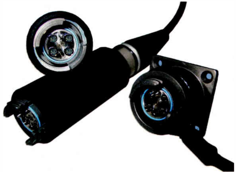
Multipin expanded beam connectors make repeat matings easy and reliable. Flush, noncontacting lenses simplify cleaning compared with pin-and-socket connectors, which tend to trap dirt.
