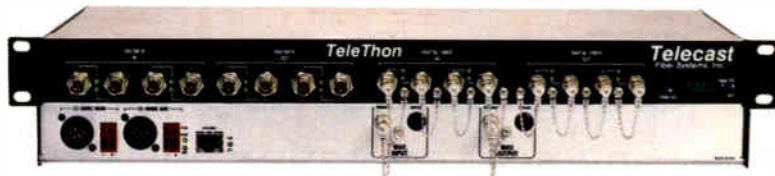
A single-unit CWDM manager converts both wideband electrical and optical signals to the appropriate wavelengths for transport on just two single-mode fibers.
