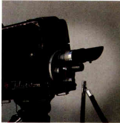
This photo of a 1950s camera shows how lenses were mounted on a turret to enable an operator to choose the appropriate focal length.
