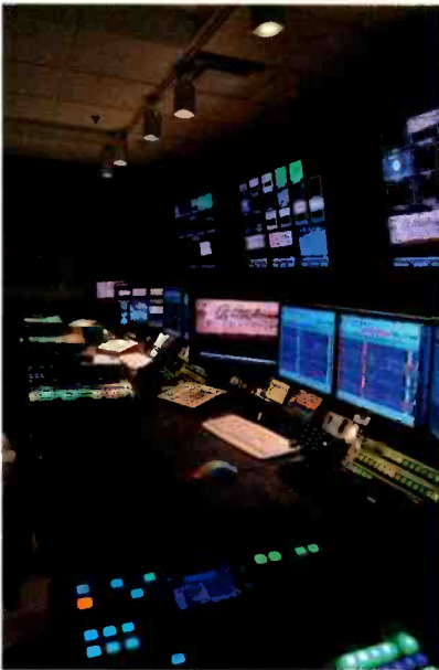
This HD/SD MC (one of four) at the Golf Channel uses an Evertz QMC switcher and MVP multiviewer software.
