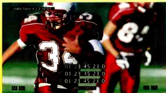
Image showing timecode and metadata overlay mode. G1-G4 indicate AES audio presence, WSS, VI, AFD and CC are present when highlighted.
