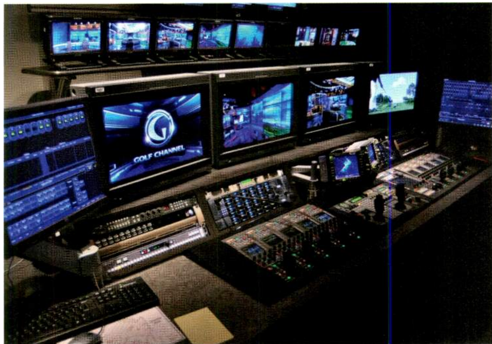
The video and camera control area contains the operations control panels for the Sony HD studio cameras. The cameras can be remotely adjusted, and the camera signals can be evaluated before going to air.
