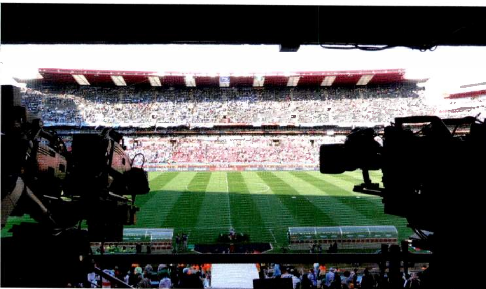
ESPN's World Cup coverage used Sony HD cameras mounted on side-by-side rigs above the field to provide the best wide-angle views in 3-D. The consensus is that side-by-side rigs work best from higher positions.
