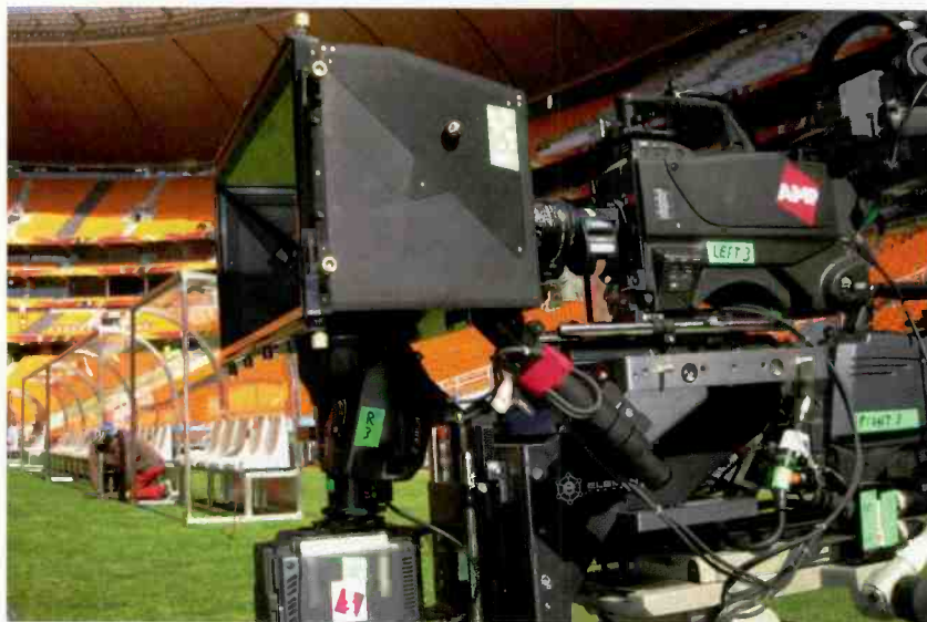
At the World Cup, Canon HJ22ex7.6B lenses were mounted on Sony HDC-1500 HD cameras inside Element Technica 3-D rigs. Beam-splitter rigs are common at most live 3-D sports productions because they can get closer to the field.
