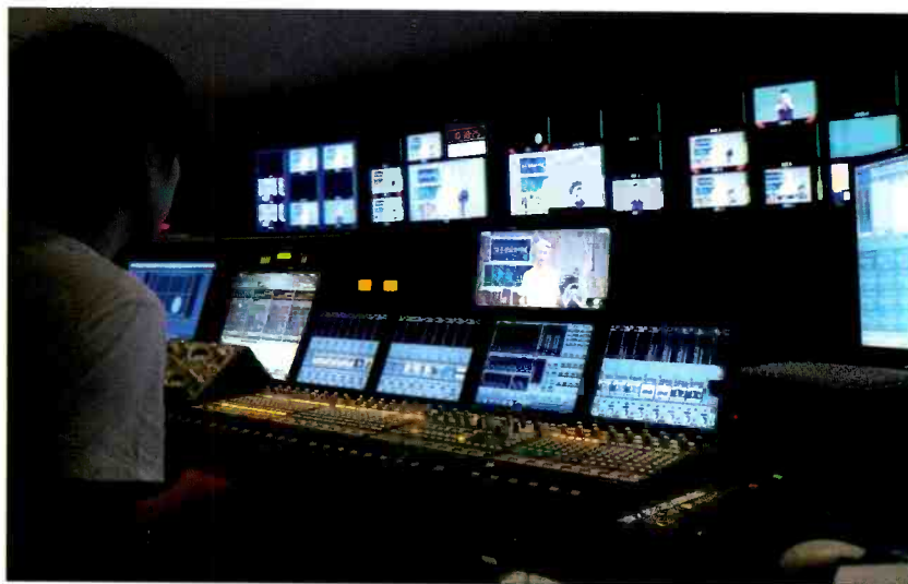
Implementing 5.1 often mandates a major equipment upgrade by facilities, as the complexity of a mix situation involving simple stereo and 5.1 surround is best accomplished in a digital production workflow.
