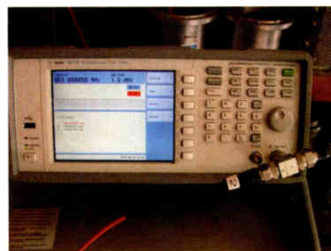
Figure 4. The signal generator displays the three stored station frequencies.
