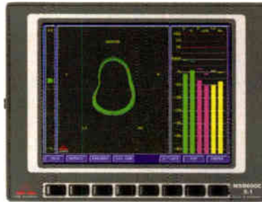
Most engineers monitor 5.1 audio by looking at a level meter or graphical display of the surround-sound environment.
