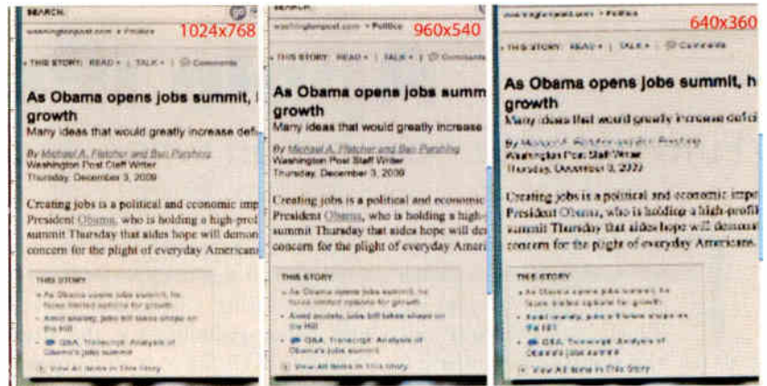
Figure 2. Shown here is video encoded at 1024 x 576, 960 x 540 and 640 x 360, and then played on the iPad.
