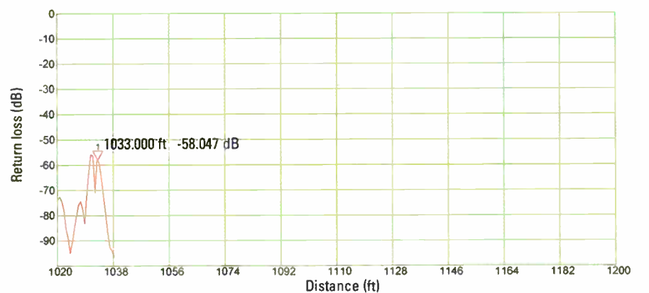
Figure 2. Initial measured time domain length difference for lower transmission line
