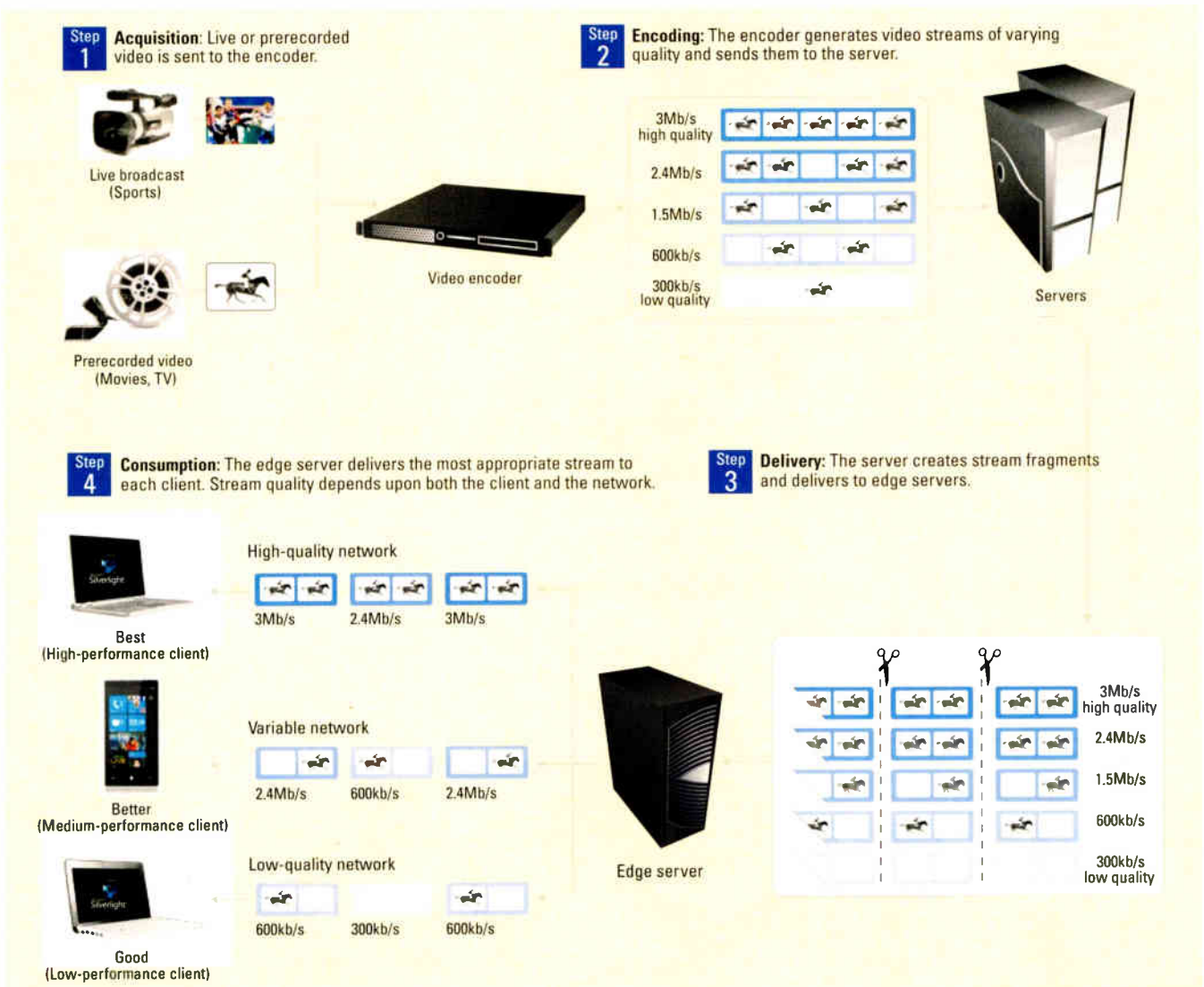
Figure 2. Microsoft IIS Smooth Streaming can adapt to changing network conditions by varying the quality of the stream.
