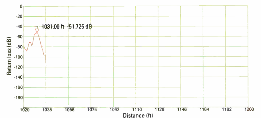
Figure 3. Initial measured time domain length difference for upper transmission line
