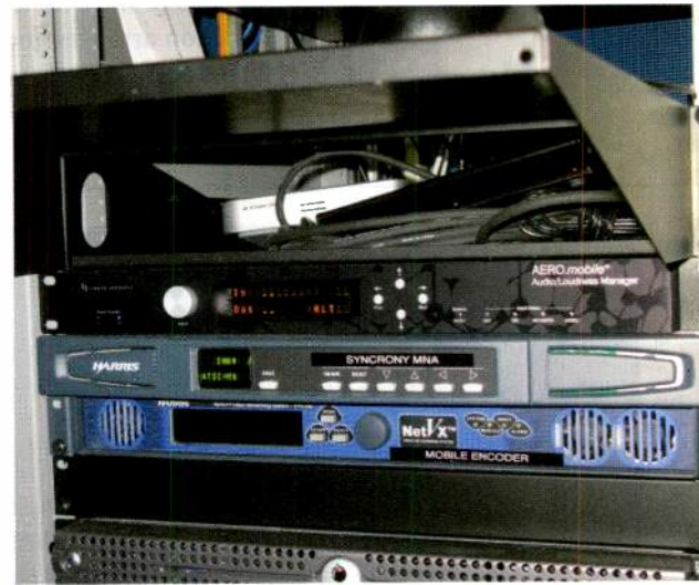
Linear Acoustic's AERO.mobile can downmix and process separate audio streams to provide controlled, intelligible results for mobile devices.
