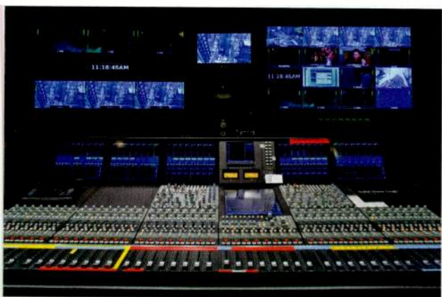
The audio control room houses a Solid State Logic C140 console mixing surface and several roll-around racking carts to accommodate a variety of outboard audio and peripheral support equipment.
