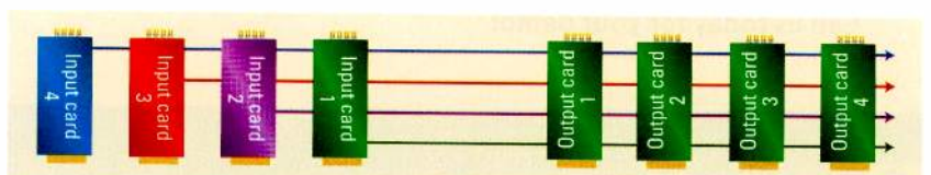
Figure 4. The daisy-chain video path architecture can be used for the communication channel.
