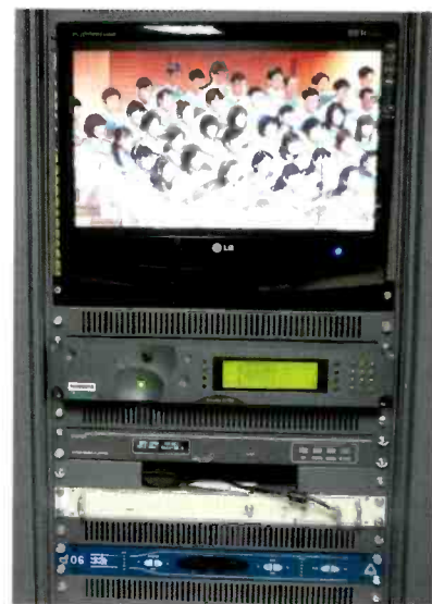
Jünger's Television Audio Processor combines audio processing and encoding in the same unit.
