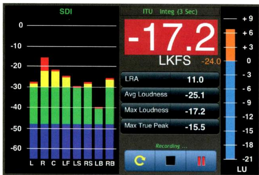
Figure 1. Pandora's layout shows both absolute loudness (left pane) and integrated loudness relative to level setting (right pane).
